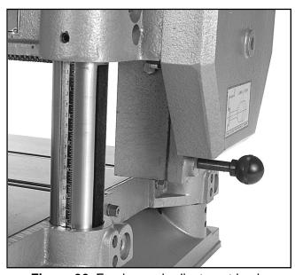
Figure 36. Feed speed adjustment knob.
